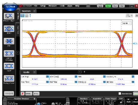
Data Rate = 2.5 Gb/s, V_{in} = 220 \text{ mV}_{pp}
