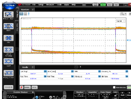
Data Rate = 100 Mb/s, V_{in} = 220 \text{ mV}_{pp}
