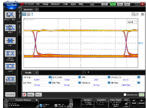
Data Rate = 1 Gb/s, V_{in} = 220 \text{ mV}_{pp}
