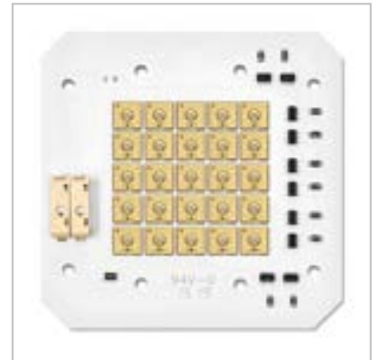
One 5x5 LED Array from Bolb provides powers up to 2.5 W.
