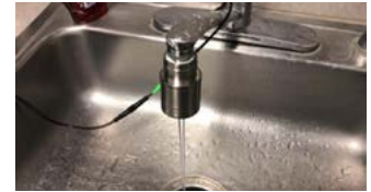
Figure 2: Water faucet (PoU) disinfection.
