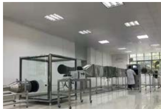
Figure 3: Testing of a 3,000 LPM air disinfectant at the Guang Zhou Institute of Microbiology, achieving a 99.96% single pass kill rate against aerosolized staph aureus.
