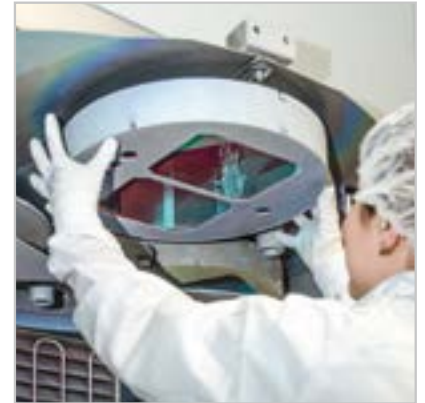
The substrates are inserted into a PIAD coating machine.
