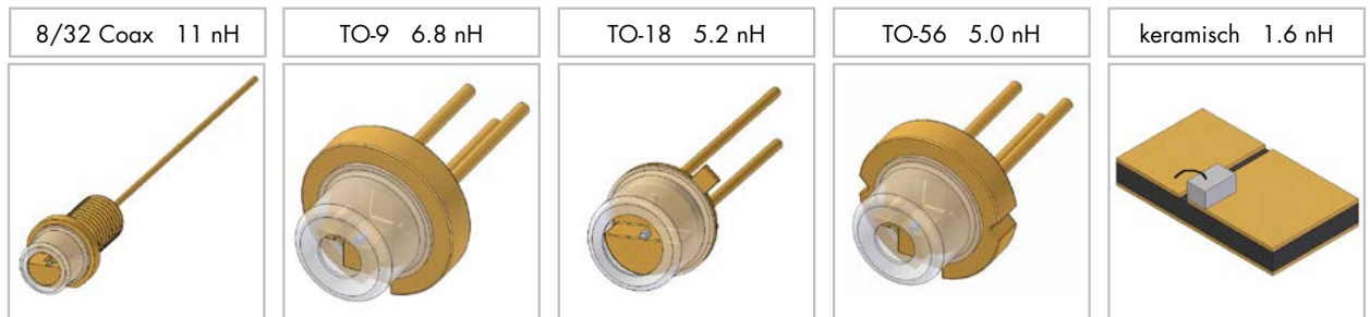
Figure 3: Different types of PLD housings and their corresponding inductances
