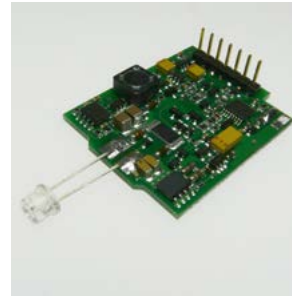
PLD in plastic housing and long pins Current rise time approx. 12 ns
