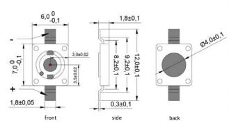
VD-0940I-400M-1A-2A0 with Substrate 1=AIN and Package A=2016 (unit: mm)
