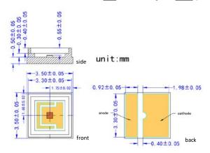
VD-0940I-400M-3E-2A0 with Substrate 3=Cu/Ag and Package E=7060 (unit: mm)
