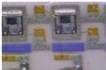
**Figure 2: Close-up of LED chip assembly**
