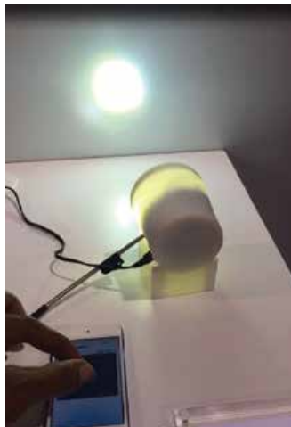
Dynamic control of beam angle with liquid crystal lens operated by a touchpad.
