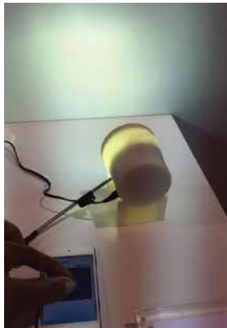
Dynamic control of beam angle with liquid crystal lens operated by a touchpad.
