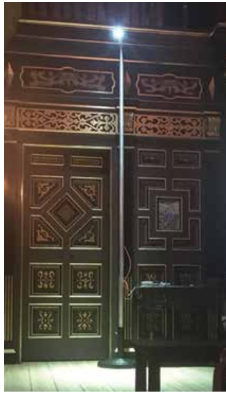
A streetlight demo with blue laser light transported by fiber to the phosphor element at top with optic.
