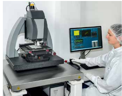
An ion-beam sputtering (IBS) coating chamber. Laser Components uses IBS coating technology to reach highest reflection and transmission values, from 248- to 3000-nm wavelength range (left). To reach the best possible results for high-quality laser optics, Laser Components controls the surface roughness by using white light interferometry (right).
